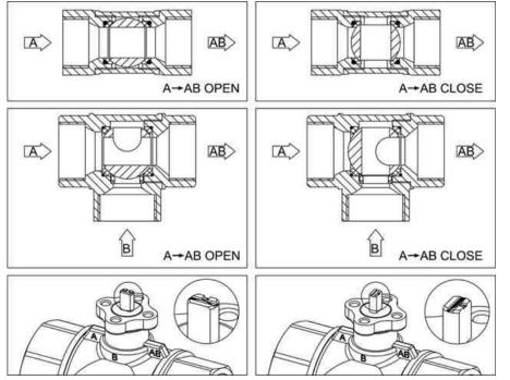
The Kv (Cv) ratings listed on above table are from port A to port AB. The flow ratings from port B to port AB are about 50% of above Kv (Cv) ratings.
