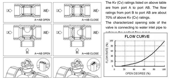
SBV02 series 2-way valve must be installed on the return pipe to reduce thermal stress on the valve ball sealing. SBV02 series 3-way valve can be used as mixing valve or diverted valve. **Please notice that the "T" mark on valve stem indicates the ports on the valve ball.**
